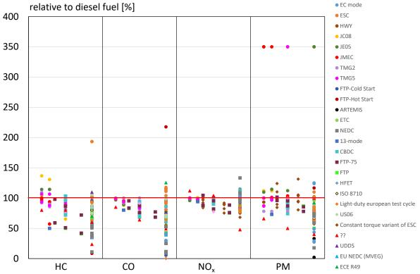
Figure 4: Overview for regulated emissions of GTL and GTL blends relative to diesel fuel. The blend proportion starts with 5% left side and goes up to 100% right side of each emission component. The single tests are coloured by the test cycles used. (Original literature is not cited in this review.)
