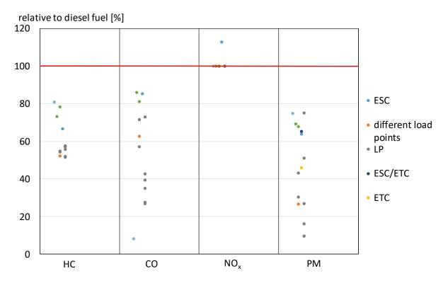
Figure 5: Overview for regulated emissions of OME<sub>3-5</sub> blends (5, 10, 15, 20, and 25% from left to right in each column) relative to diesel fuel. The single tests are coloured by the test cycles used. (Wang et al. 2015, Liu et al. 2017, Liu et al. 2016, Feng et al. 2016, Lumpp et al. 2011 and Härtl et al. 2015).
