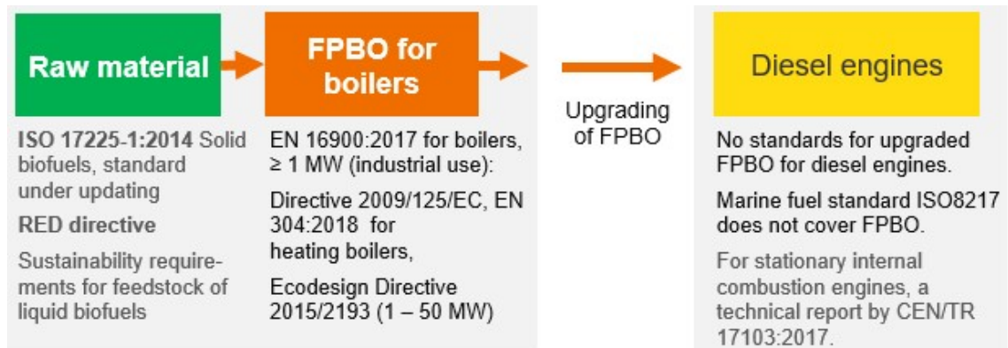
Figure 4-1. Status of standardisation of the FPBO and upgraded FPBO.
