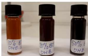
Figure 4-2. Blends with DMB containing 10%, 30% and 50% of SDPO [4-17].
