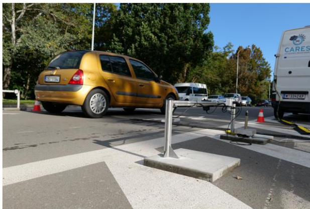
Figure 42: RES type 2 measurements for the detection of particle high-emitting diesel cars in Prague/Brno 2022. Of the 16 out of 17 cars with high PN emissions according to the RES measurements, 13 cars were confirmed as true high PN emitters and three cars as suspicious high PN emitters in the roadside idle PN test. Only one car was a false failure according to the RES measurements [53].
