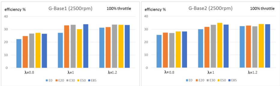
Fig. 5.19 Thermal efficiency of Ricardo Hydra GDI research engine at 2500 rpm operation with full throttle position
