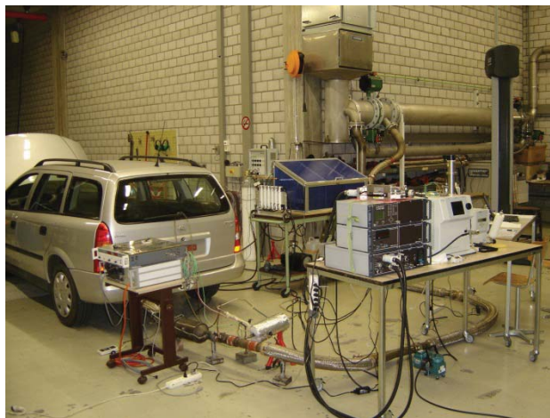
Figure 2: The exhaust exposure system, located at the Bern University for Applied Sciences in Nidau Prof. J. Czerwinski's lab. A) test vehicle, B) exhaust sampling, C) characterization of the particulate exhaust fraction D) cell exposure system.
