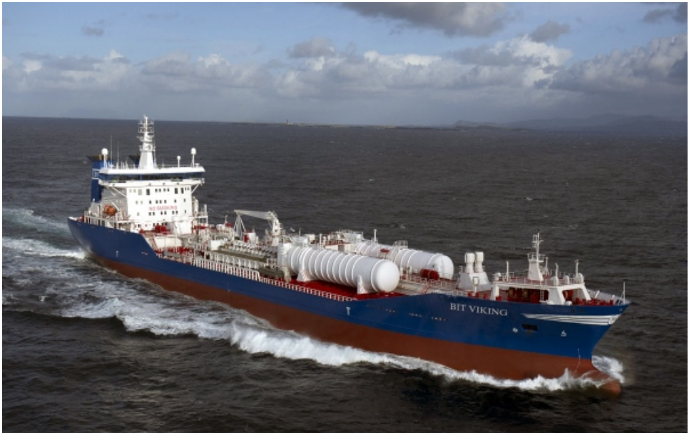
Figure 20. “Bit Viking” with LNG Fuel Tanks on the Main Deck
