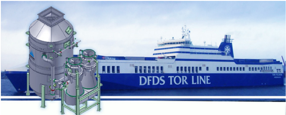
Figure A-4. Ficaria Seaways Equipped with Presumably World’s Largest Retrofit Scrubber in 2009 (Source: Alfa Laval)
