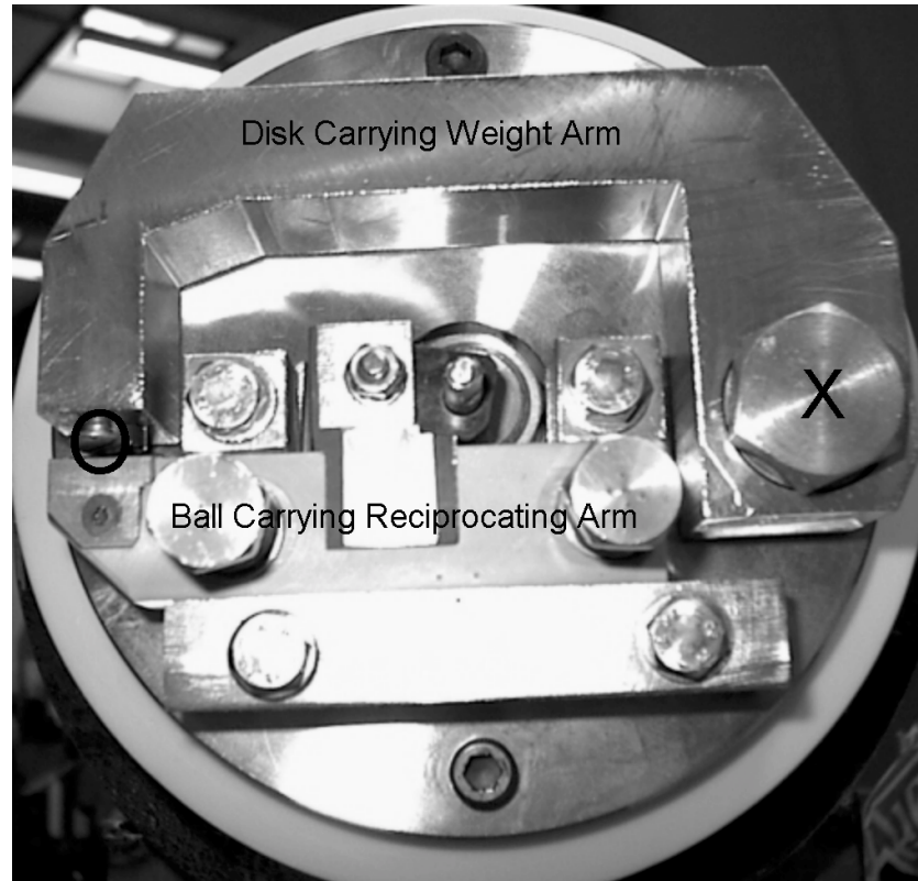
Figure A1: The inside of the MFPRR.
