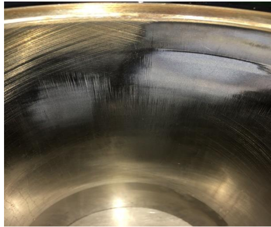
Figure 5.15 Bore morphology of corrosion-resistant gray cast iron cylinder liner after 1500 hours of operation
