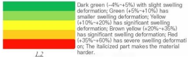
Figure 1.21 Analysis of the Effect of Different Methanol Concentrations on Different Rubber Materials
