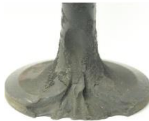
Photo of exhaust valve erosion
