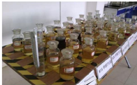
Figure 1.22 Analysis of the Effect of Different Methanol Concentrations on Different Plastic Materials
