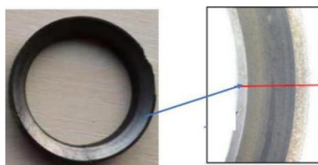
Figure 3.9. Morphology and contact broadband of exhaust valve seat ring
