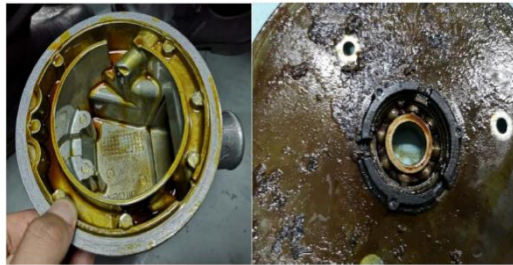
Figure 8.5 Corrosion of Oil Gas Separator for Reliability of Heavy Duty Methanol Engine
