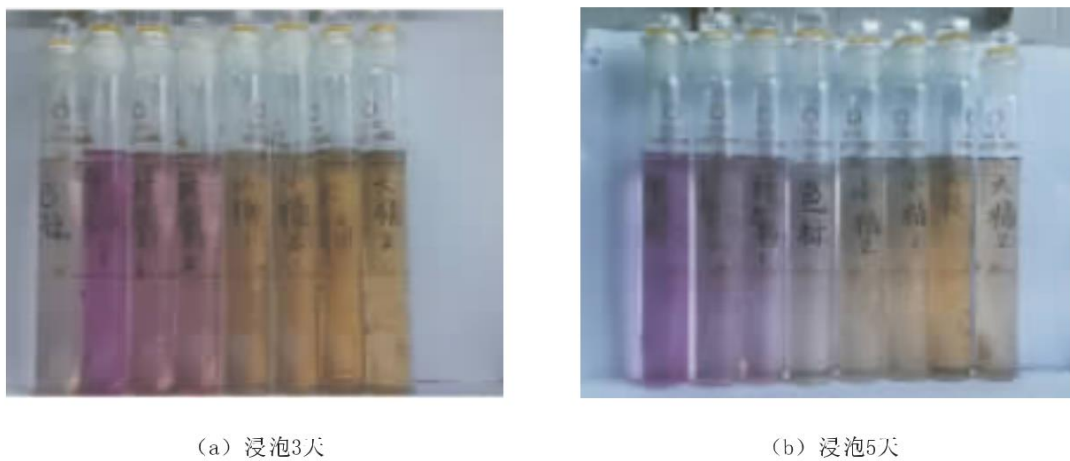
Figure 1.16 Color comparison of methanol samples with potassium permanganate added after different soaking times
