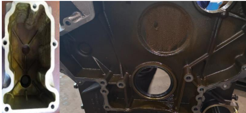
Figure 8.4: Oil sludge situation for reliability of heavy-duty methanol engines
