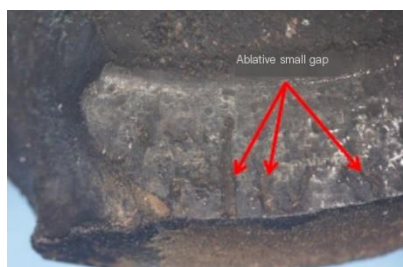
Figure 3.3 Morphology near the ablation area of the exhaust valve
