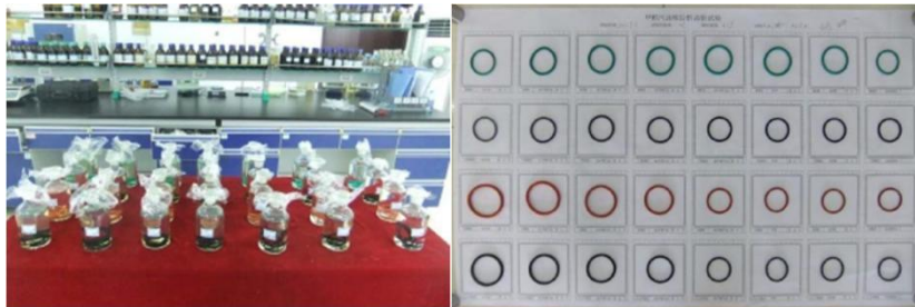
Figure 1.20 Immersion of different rubber materials in solutions with different methanol concentrations
